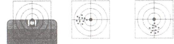
□ To aim the left, turn with a right-angled screwdriver the right screw on the rear sight rightward. It would be deflected to the left if rotate it leftward.
