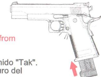
□ While loading the magazine, push it inward to the bottom till a "click" sound is heard. Press the magazine release catch, the magazine will fall off from the stock.
