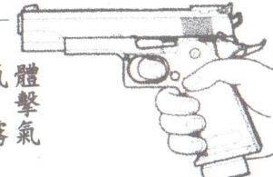
After a long and continued firing practice, the low temperature of the magazine will cause a reduced gas pressure as well as the low Velocity of bullet. It is a normal condition, not a trouble. Never practice the reverse firing because which action cause the gas can't evaporate and the vapor easy to damage the parts.
