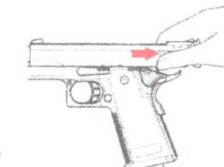
□ Pull the slide backward to a specific position, then release and let the slide moving forward to load the bullet in the firing chamber, and retain the hammer at the rear position, ready for firing.
